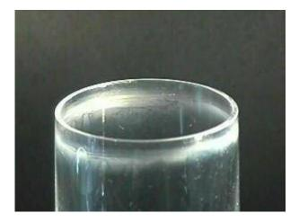
Figure 1: Local clouding on the rim Source: Glastechnische Tagung Leipzig 2003
